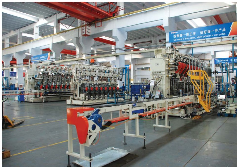
Machines have been introduced to the Sanjin portfolio that are more productive and capable of making high quality bottles and jars, including 10-section triple gob and 12-section double gob machines.
